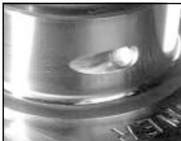
The unique teardrop scoop and exclusive Crower "straight-shot" oiling system increases critical oil flow from the main bearings to the rod bearings.
