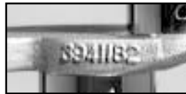
The forging I.D. number on the Crower Stock-Plus and Pure-Stock is GM part number “1182” indicating stock.
